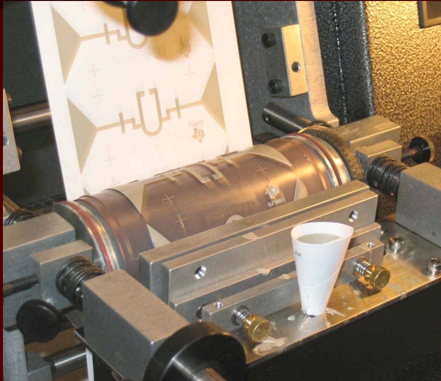
Antenna Printing Process on Labels
