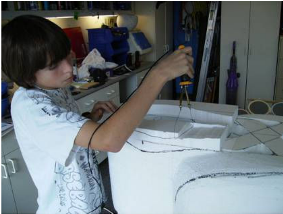
Carving Foam with hot wire
