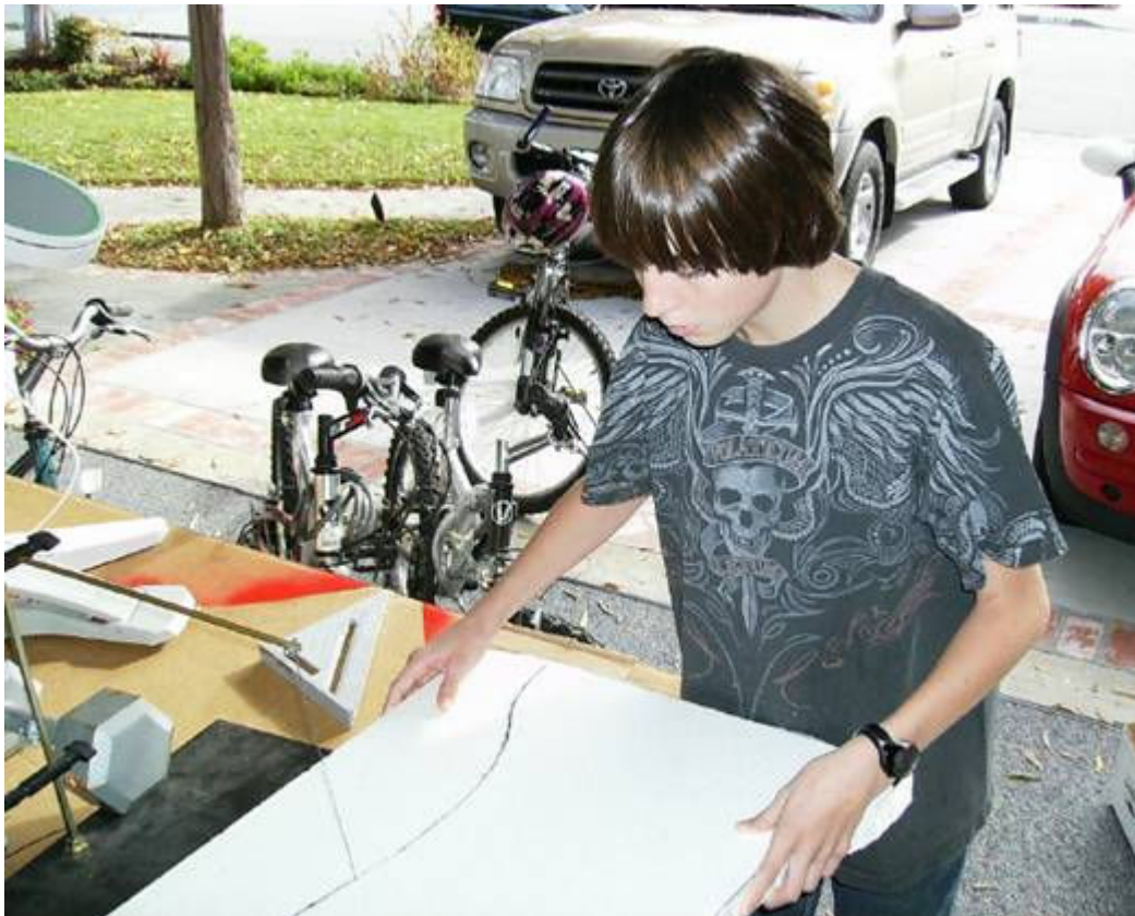
Using hotwire to cut EPS foam sheets
