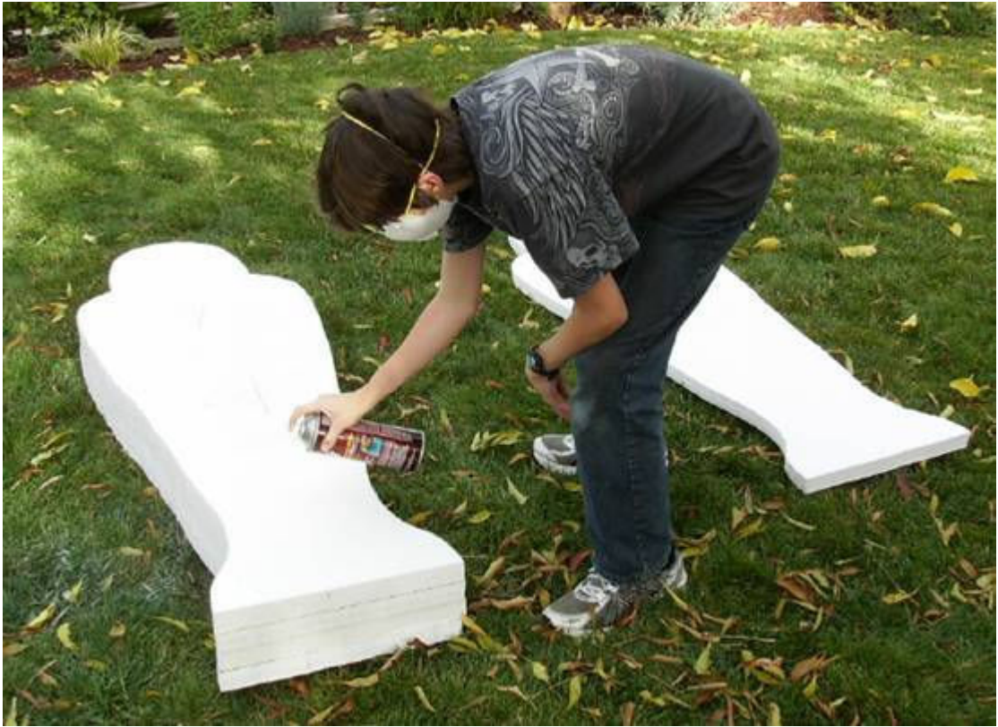
Bonding piece together with contact cement spray glue (3M #77)
