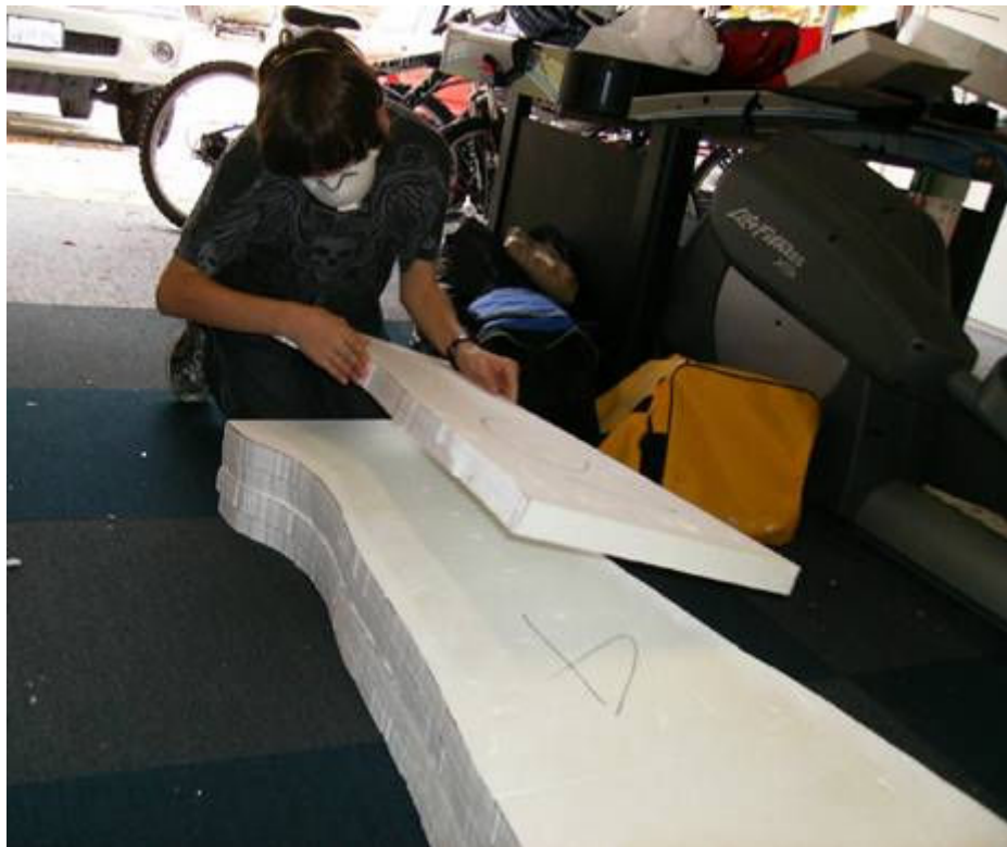
Positioning foam piece must be perfect first time – bonds instantly
